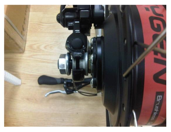
**Step 5.**Securing the front wheel is very important. The locking nuts should be well tight with a minimum torque of 12Nm.
