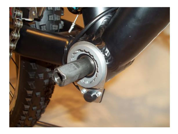
The speed sensor should be located under the bottom bracket shell.
