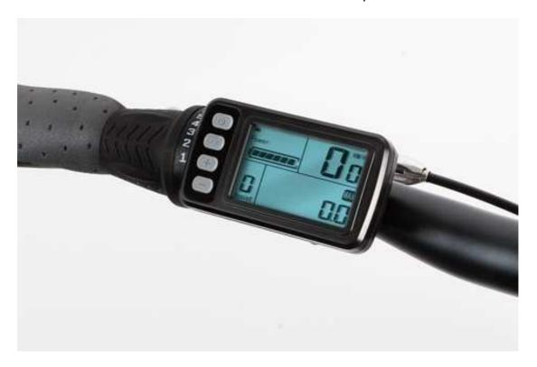
Fitting the throttle and the power setting buttons will depend on the type of the bike and this has to be tried by each user. Throttle can be located on either left or right hand side of the handlebars. If fitted on the left the thumb twist will have to move forward then.
